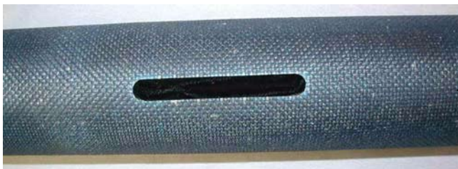
FIBER GLASS SLEEVE THE PHOTO SHOWS THE KEYED SLOT THAT HOLDS SLEEVE IN PLACE
